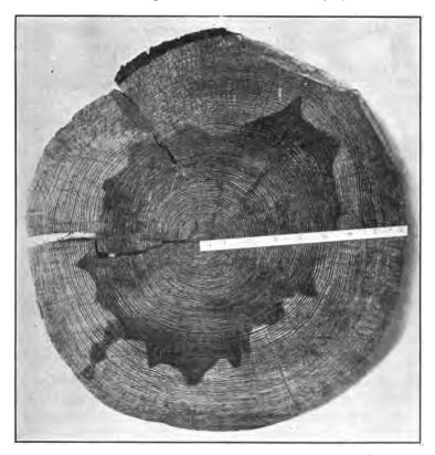
Fig. 30.—Cross section of longleaf-pine tree showing sapwood and heartwood.
